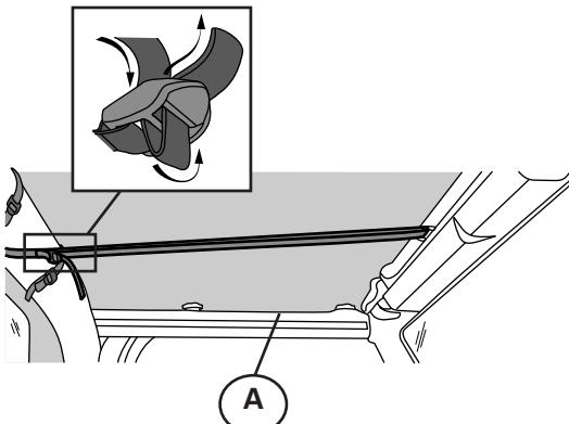
**8** Thread the strap through the footman loop above the windshield. Pull the end of the strap back and thread it through the buckle. Pull it tight.
