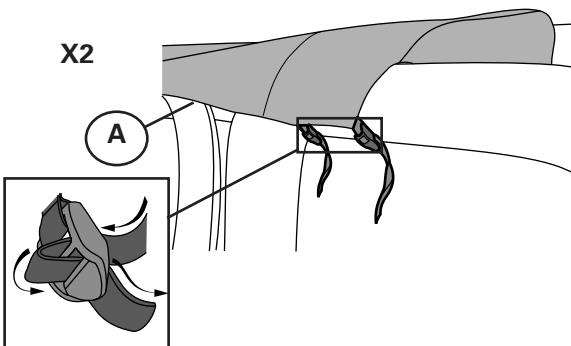
**9** Wrap the straps on the rear of the Sunbonnet around the speaker pods, two straps on each side. Thread them through the buckles.
