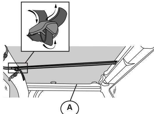
**7** Thread the strap through the footman loop above the windshield. Pull the end of the strap back and thread it through the buckle. Pull it tight.
