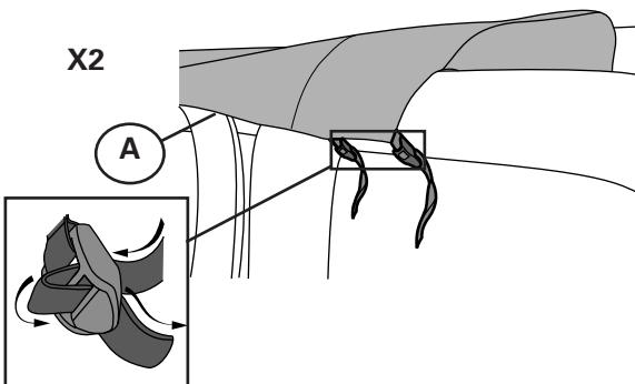
**8** Wrap the straps on the rear of the Sunbonnet around the speaker pods, two straps on each side. Thread them through the buckles.
