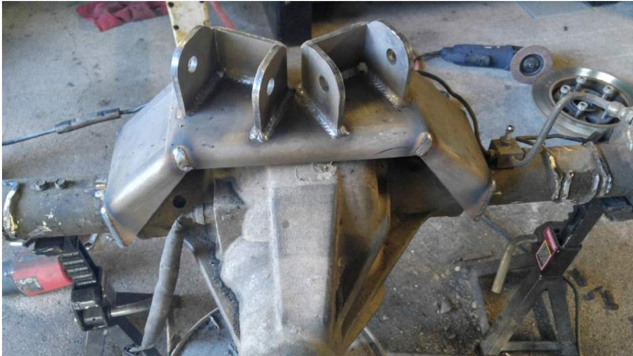
Here you can see where the upper control arm brackets were cut off the axle and the truss were welded to the axle. I was running short on time and didn't grind the old brackets smooth, but I will when I get back from my Colorado trip. Prior to welding this bracket to the axle Marty recommended I grind the top of the axle housing I believe a 1/16, but don't remember the exact measurement. See picture below.
