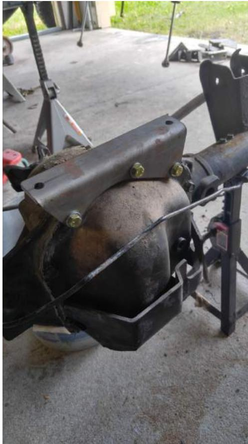
You can see how I have the brake line in front of the diff cover for now. The bracket you see on top of the diff cover is what you will use to align the rear truss. I put this bracket on and tightened the bolts only tight enough to hold it in place but still able to move the bracket.
