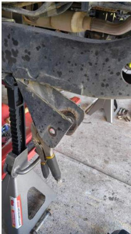
This was the most time consuming process to cut all control arm brackets off the frame and grind everything smooth.
