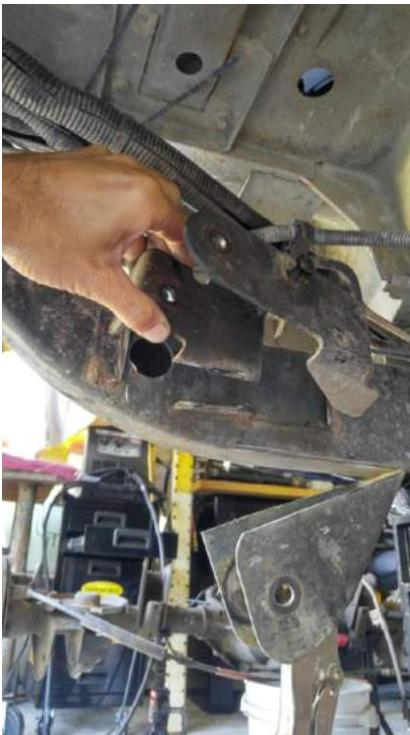
Be careful cutting around brake lines, locker lines and electrical lines.
