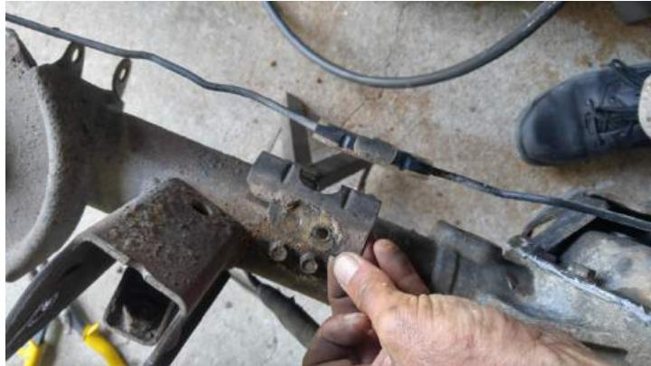
I removed this bracket that holds the brake line to the axle. It may not seem the brake line will have enough to be rerouted, but if you carefully work with the line it will bend around the diff cover.
