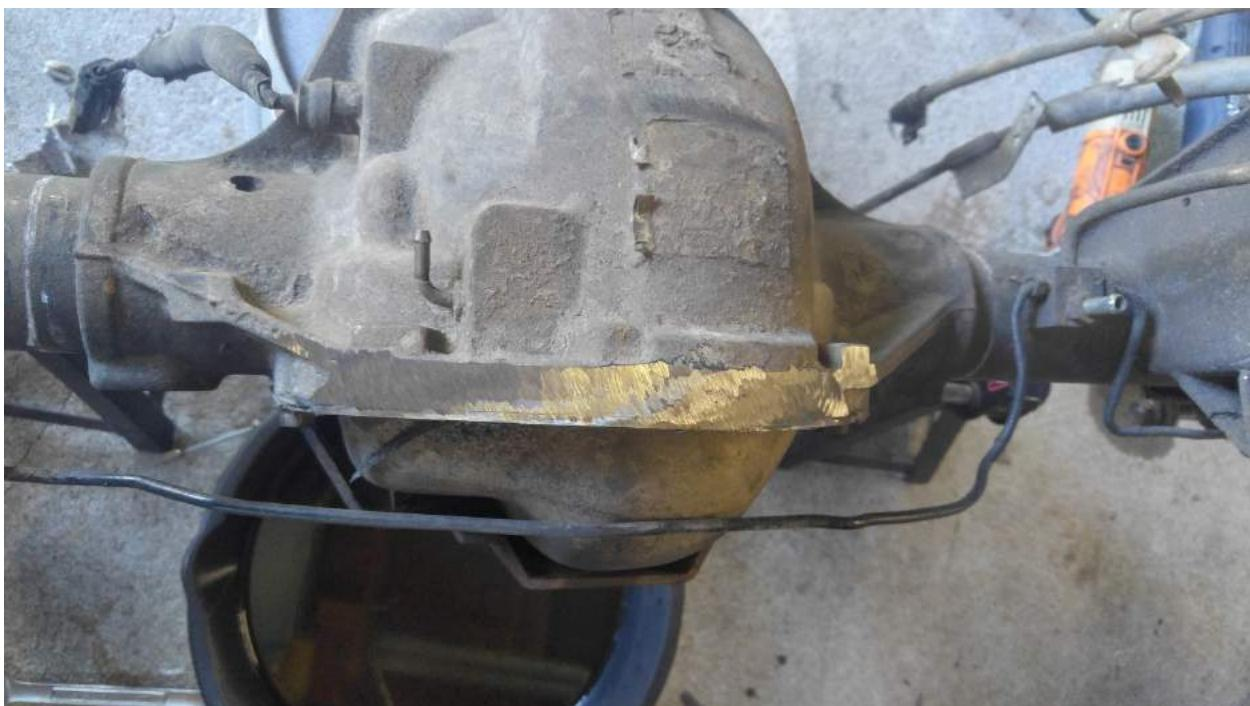
Once I got the rear truss welded on and upper control arm brackets removed from the axle I began working on the front axle.
