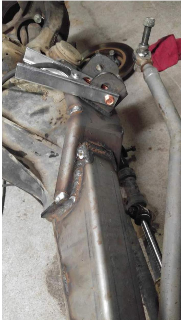
I will put the documents that I received from Marty for the placement of the brackets that still need to be welded to the frame. Be sure to prep the frame and grind everything down to bare metal for good weld penetration. Also these documents will give you an initial setup for control arm lengths.
