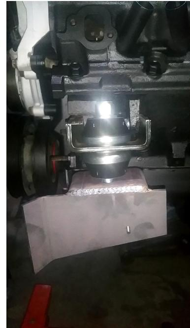
case, and place the drive shaft in. From there you can cut the dowels off the motor mounts (takes less than a few seconds with a harbor freight cut off) and tack the motor mounts in, pull the drivetrain, and weld them in place. This will allow you to keep your driveshaft. However, it will make it so that you will more than likely have to hammer in your firewall
