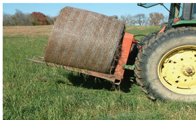
Figure 10 - Raise Carrier to a Consistent Height
