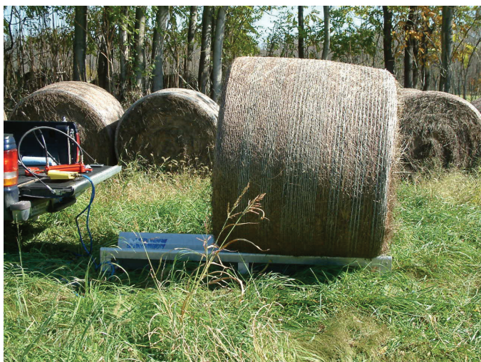
Figure 2 - Weighing Bale on Livestock Scale
