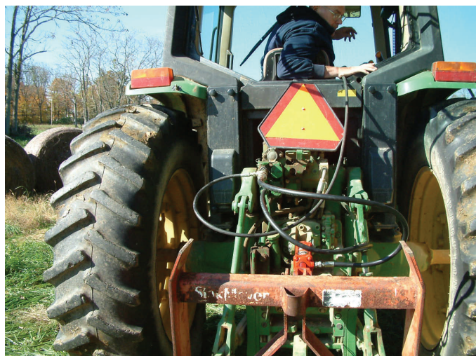
Figure 8 - Rear view of Cylinder as Top Link
