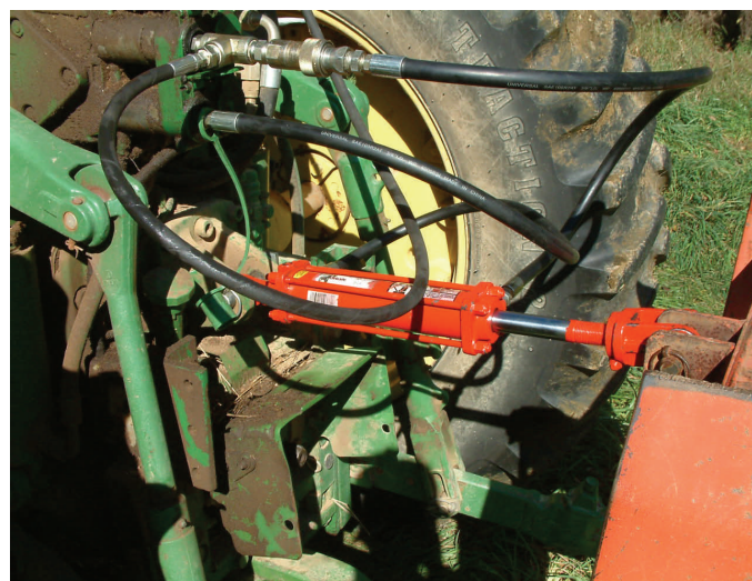
Figure 9 - Side View of Cylinder as Top Link
