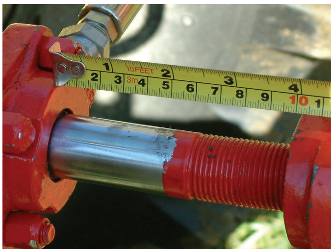
Figure 11- Let out the Cylinder to a Consistent Length
