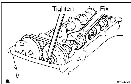
(d) Fix the camshaft with a spanner and so on, then tighten the camshaft timing gear set bolt.
