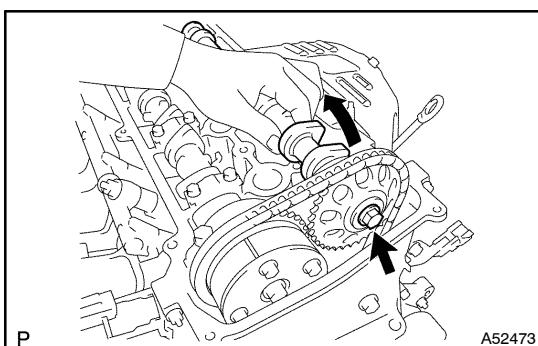
(c) Raising the camshaft, remove the set bolt.
