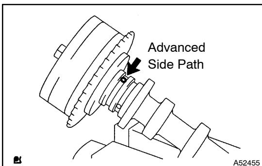
**13. REMOVE CAMSHAFT TIMING GEAR ASSY**
