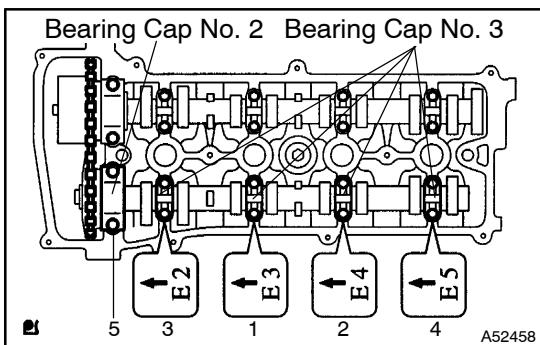
(c) Examine the from marks and numbers and tighten the bolts in the sequence shown in the illustration.
