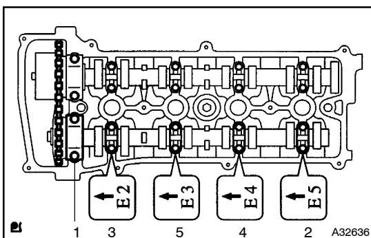
(b) Loosen the camshaft bearing cap bolts on No.2 camshaft in the sequence shown in the illustration in several passes, and remove the caps.
