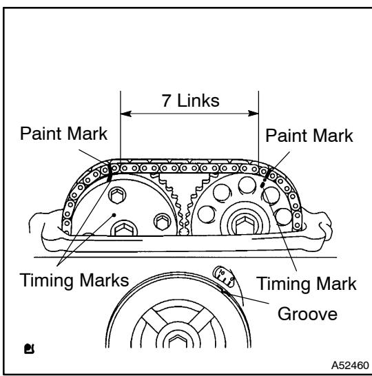
(e) As shown in the illustration, check the match marks on the timing chain and camshaft timing sprockets and the alignment of the pulley groove with timing mark of the chain cover.
