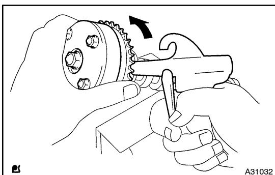
(c) Put air pressure into the oil path with 150 kpa (1.5 kgf/cm<sup>2</sup> 21 psi), and turn the camshaft timing gear assembly to the advance direction (counterclockwise) by force.
