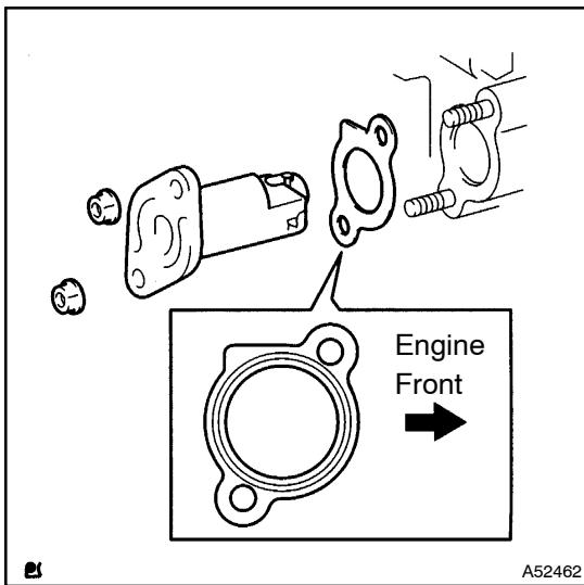
(b) Install a new gasket and chain tensioner with the 2 nuts.
