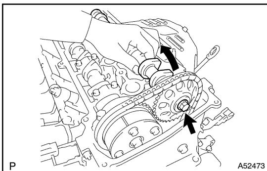
(b) Raising the camshaft, tighten the set bolt temporarily.
