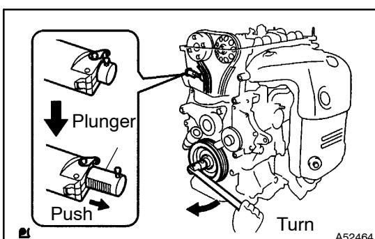
(d) Turn the crankshaft clockwise, and check that the plunger is pushed by the plunger.
