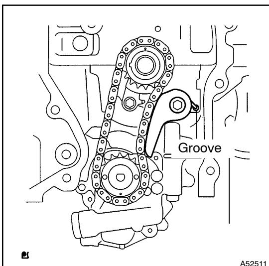
(f) Insert the damper spring into the adjusting hole, and install the chain tensioner plate by a bolt.
