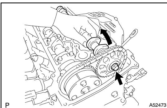
(f) Raising the camshaft, remove the set bolt.
