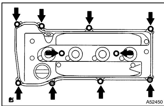
7. REMOVE CYLINDER HEAD COVER SUB-ASSY
