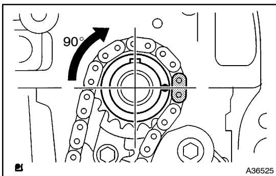
(i) Rotate the crankshaft clockwise  $90^\circ$ , and align the crankshaft key with the top.
