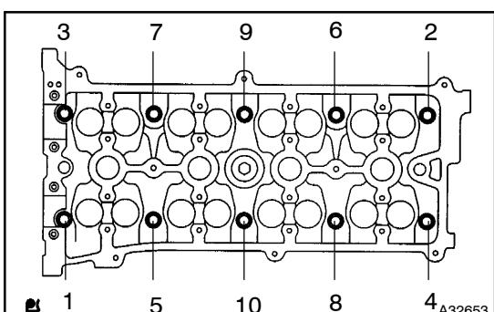
**34. REMOVE CYLINDER HEAD SUB-ASSY**
