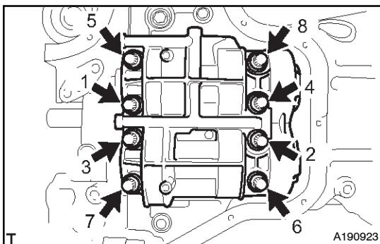
(f) Temporarily tighten 8 bolts in the several passes as the sequence shown, and fully tighten with specified torque.
