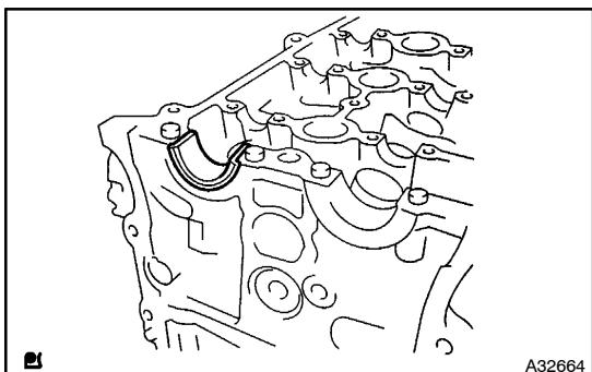
**32. REMOVE CAMSHAFT BEARING NO.2**
