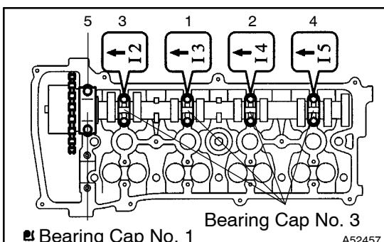
(o) Examine the front marks and numbers and tighten the bolts in the order shown in the illustration.
