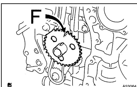
**79. INSTALL CRANKSHAFT POSITION SENSOR PLATE NO.1**
