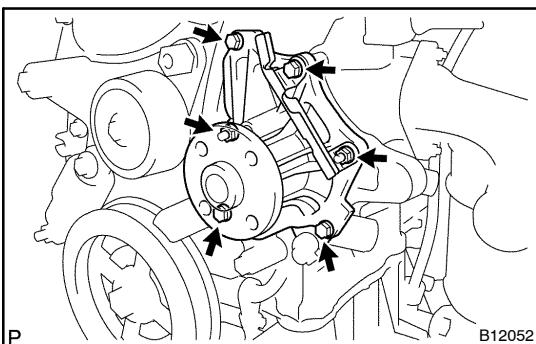
(c) Install the water pump assembly with 4 bolts and 2 nuts.
