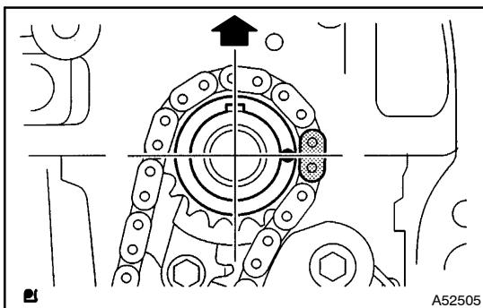
(2) Using the crankshaft pulley bolt, turn the crankshaft and set the set key on the crankshaft upward.
