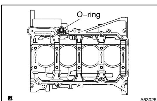
(b) Install a new O-ring the place shown in the illustration.
