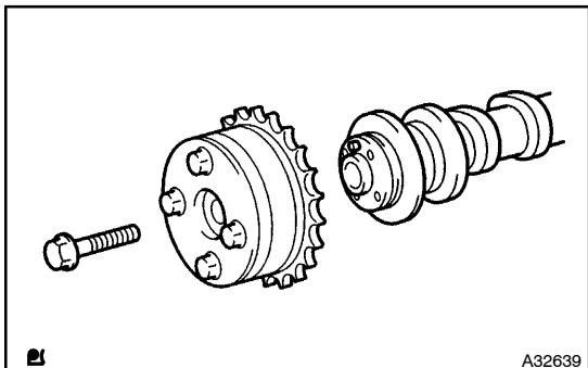
(d) Remove a fringe bolt of camshaft timing gear assembly.
