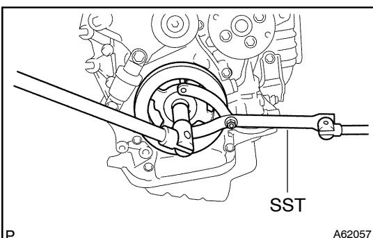
(b) Using SST, tighten the set bolt (TMMK made).
