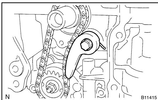
(c) Remove bolt and a chain tensioner plate.
