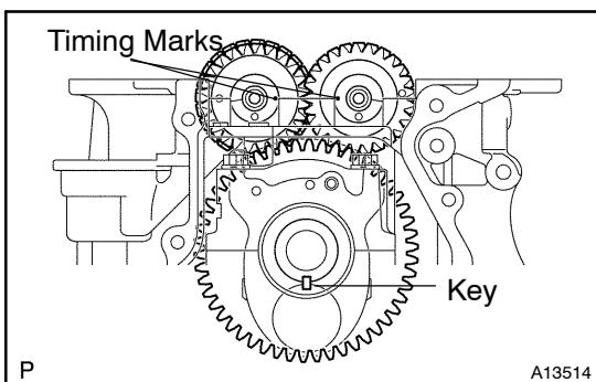
(e) Confirm that timing marks of the balance shaft are matched as shown in the illustration when the key groove is at 6 o'clock position.
