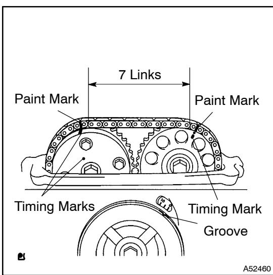
(t) As shown in the illustration, check the matchmarks on the timing chain and camshaft timing sprockets and the alignment of the pulley groove with timing mark of the chain cover.
