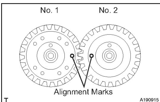
(c) Align the alignment marks of the No. 1 and No. 2 balance shaft as shown in the illustration.
