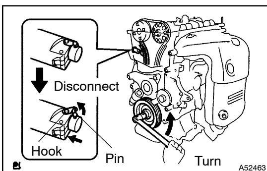
(c) Turn the crankshaft counterclockwise, and check the plunger knock pin is disconnected from the hook.
