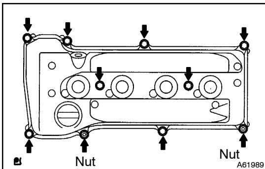
(c) Install the cylinder head cover with the 8 bolts and 2 nuts.
