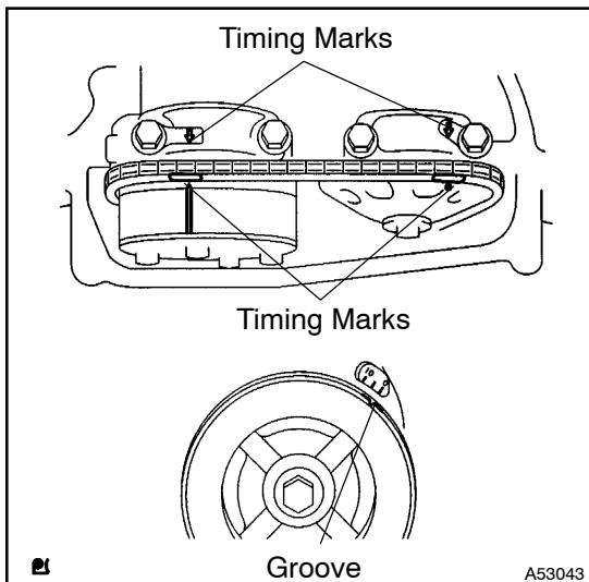
10. REMOVE CRANKSHAFT PULLEY
