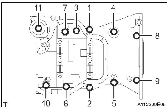
(d) Install the 11 bolts in the several passes as sequence shown in the illustration.
