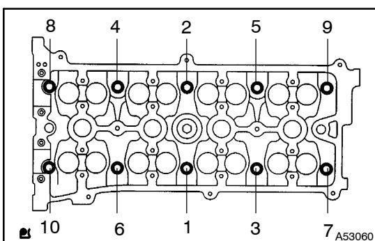
(c) Using a 10 mm bi-hexagon wrench, temporarily tighten each bolts in the several passes, as the sequence shown in the illustration, and fully tighten with specified torque.
