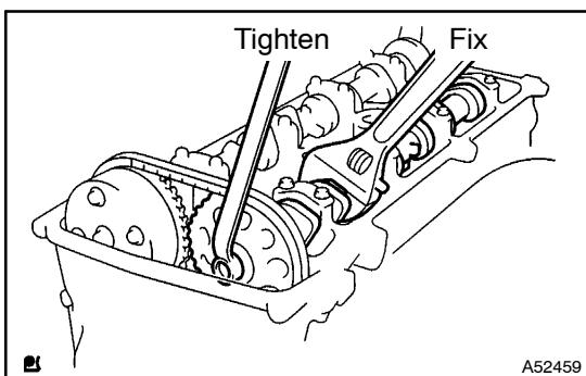
(s) Fix the camshaft with a spanner and so on, then tighten the camshaft timing gear set bolt.
