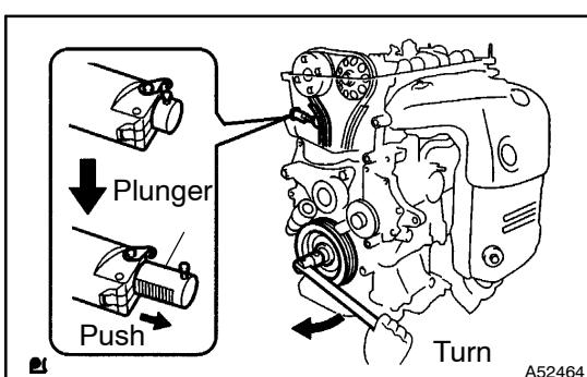
(d) Turn the crankshaft clockwise, and check the plunger is pushed by the plunger.
