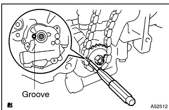
(g) Align an adjusting hole of the sprocket with the groove of the oil pump.
