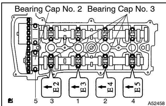
(r) Examine the front marks and numbers and tighten the bolts in the sequence shown in the illustration.
