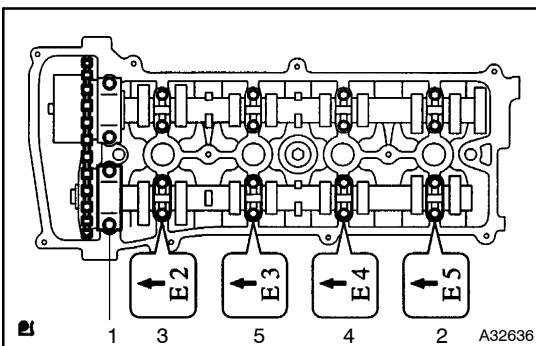
(e) Loosen the camshaft bearing cap bolts on No. 2 camshaft in the sequence shown in the illustration in several passes, and remove the caps.
