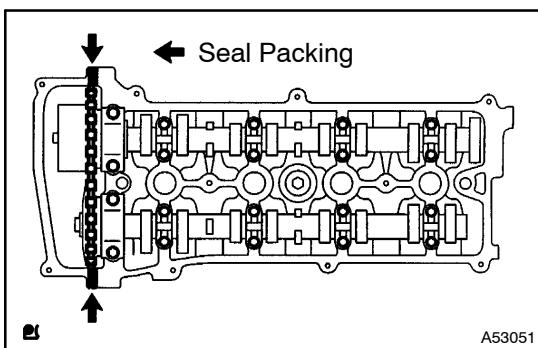
(b) Apply seal packing to 2 locations as shown in the illustration.
