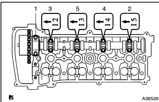
(i) Loosen the camshaft bearing cap bolts on camshaft in the sequence shown in the illustration, in several passes, and remove the caps.
