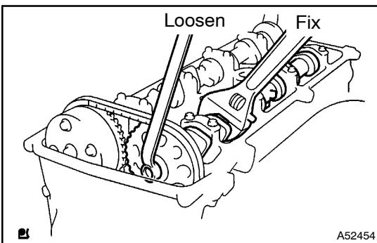
(d) Fix the camshaft with a spanner and so on, then loosen the camshaft timing gear set bolt.
