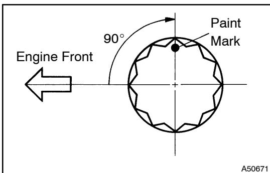
(g) Mark the front side of each balance shaft housing bolt head with paint.
