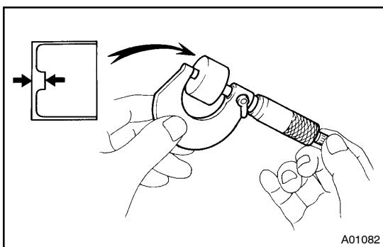
(l) Using a micrometer, measure the thickness of the removed lifter.
