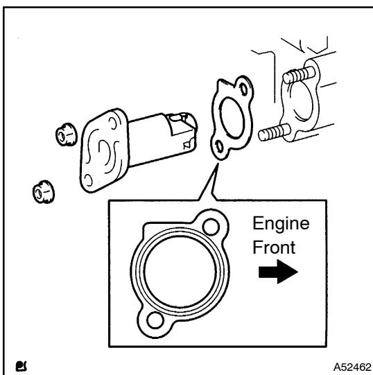
(b) Install a new gasket chain tensioner with 2 nuts.
