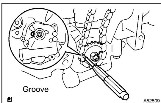
(b) Put a bar ( $\phi 4$  mm) in the adjusting hole of the oil pump drive shaft gear to lock in position, and remove a nut.
