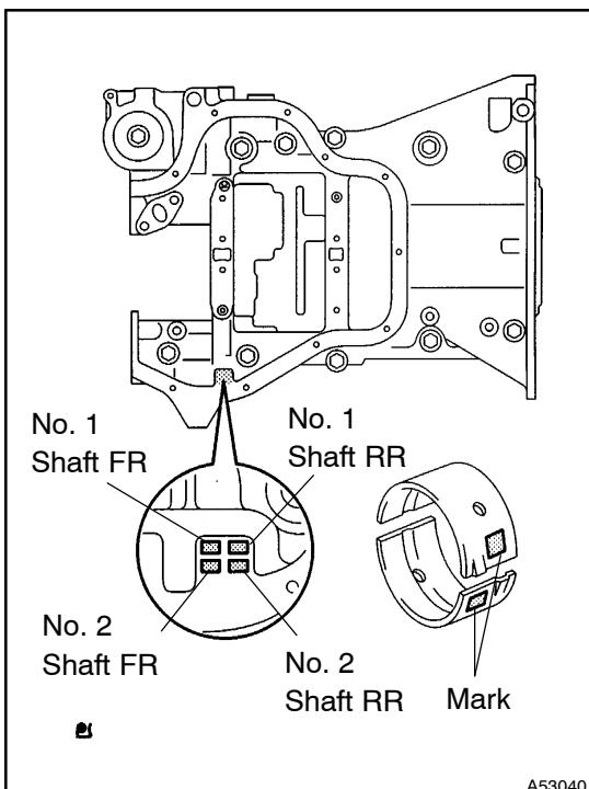
(i) If the clearance is greater than maximum, replace the bearing. If necessary, replace the balance shaft.
