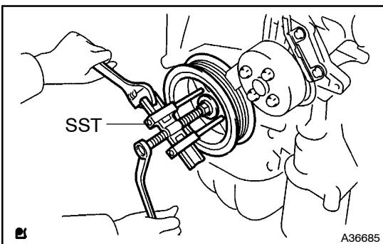
(2) Using a pulley set bolt and SST, remove the crank-shaft pulley.
