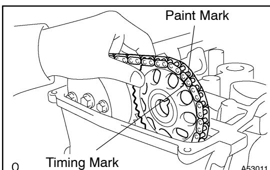
(p) Put the camshaft No. 2 on the cylinder head with the painted links of chain aligned with the timing mark on the camshaft timing sprockets.
