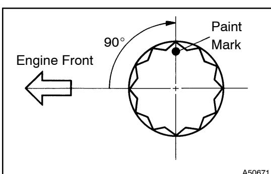
(e) Mark the front side of each balance shaft housing bolt head with paint.
