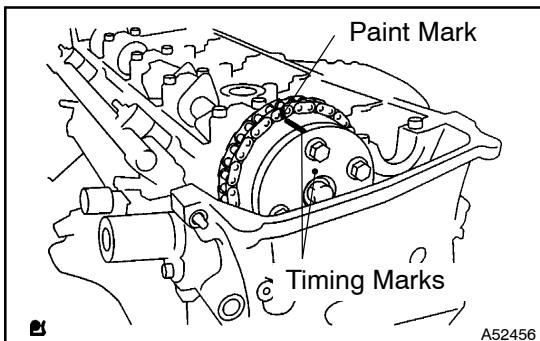
(n) Install the timing chain on the camshaft timing gear, with the painted links aligned with the timing marks on the camshaft timing sprockets.
