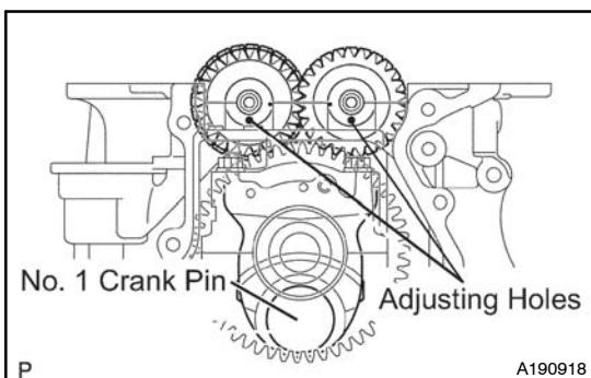
(c) With the No.1 crank pin of the crankshaft placed, at 6 o'clock position, install the No. 1 and No. 2 balance shaft and the adjusting hole as shown in the illustration.
