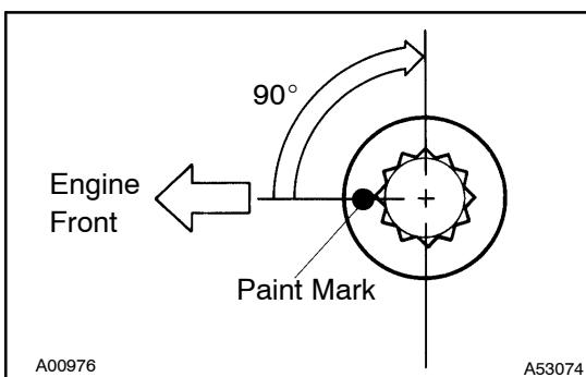
(d) Mark the front side of each cylinder head bolt with paint.
