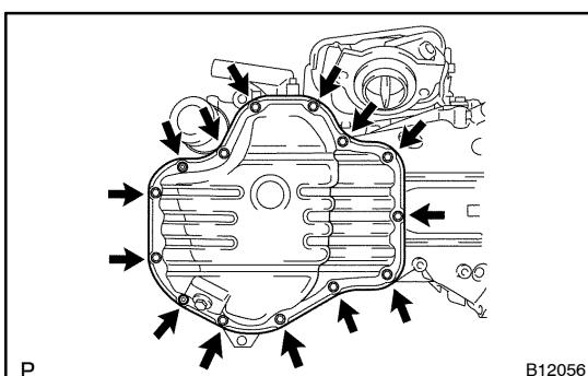
(c) Install the oil pan with the 12 bolts and 2 nuts.
