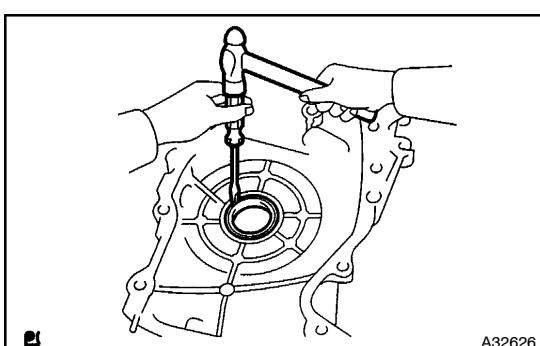
**18. REMOVE TIMING GEAR CASE OR TIMING CHAIN CASE OIL SEAL**
