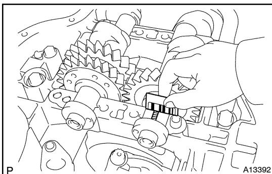
(h) Remove the balance shaft housing, and measure the plastigage at its widest point.
