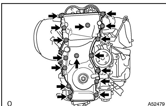
**17. REMOVE TIMING CHAIN OR BELT COVER SUB-ASSY**
