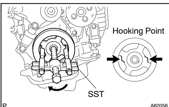
(2) Using SST, remove the crankshaft pulley.
