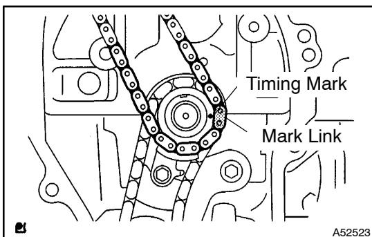
(b) Align the mark plate (blue or orange colored link) with the timing mark of the crankshaft timing gear.
