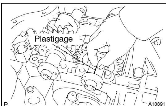
(b) Lay a strip of plastigage across each journal, and install the balance shaft housing.
