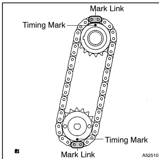
(c) Align the mark links (yellow colored links) with the timing marks of gear as shown in the illustration.
