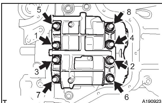
(d) Temporarily tighten 8 bolts in the several passes, in the sequence shown, and fully tighten with specified torque.
