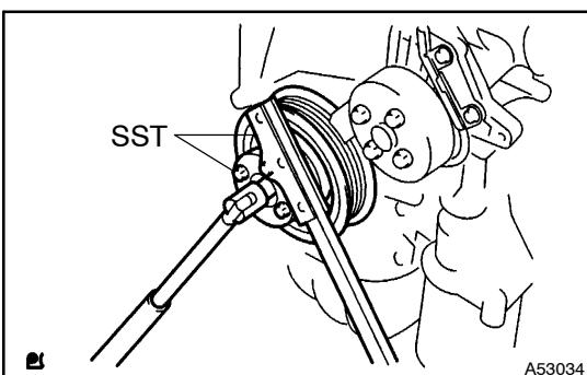
**87. INSTALL CRANKSHAFT PULLEY**
