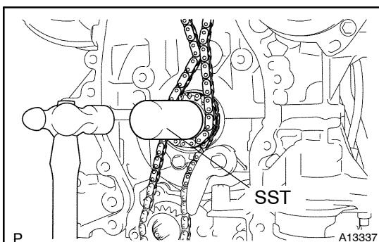
(c) Using SST, install the sprocket.
