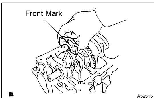
(f) Check that the front mark of the connecting rod cap is facing in the correct direction.
