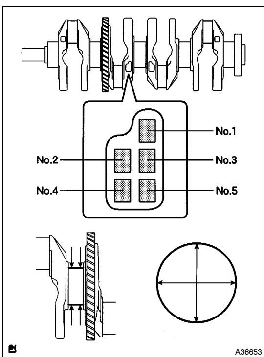
(b) Using a micrometer, measure the diameter of each main journal.
