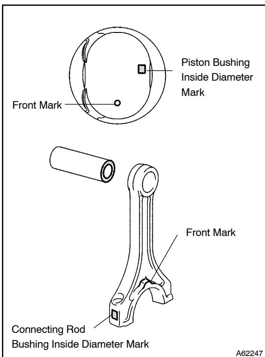
(e) If the oil clearance is greater than maximum, replace the connecting rod. If necessary, replace the piston and piston pin as a set.
