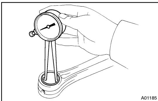
(c) Using a caliper gauge, measure the inside diameter of the connecting rod bushing.
