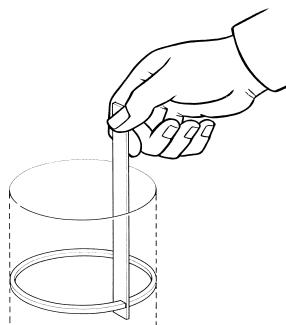
(b) Using a feeler gauge, measure the end gap.
