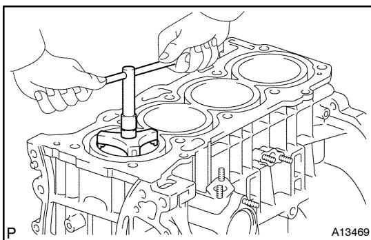
**3. REMOVE PISTON SUB-ASSY W/CONNECTING ROD**
