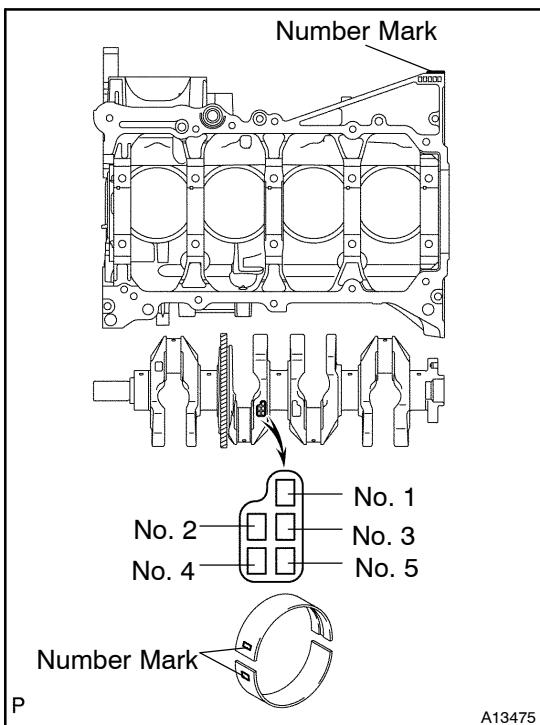
(o) If using a standard bearing, replace it with one having the same number. If the number of the bearing cannot be determined, select the correct bearing by adding together the numbers imprinted on the cylinder block and crankshaft, then selecting the bearing with the same number as the total. There are 4 sizes of standard bearings, marked "1", "2", "3" and "4" accordingly.
