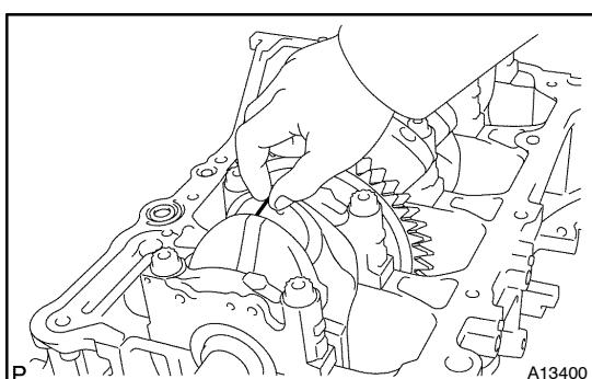
(e) Lay a strip of plastigauge on the crank pin.
