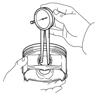
(b) Using a micrometer, measure the piston pin diameter.
