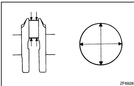
(d) Using a micrometer, measure the diameter of each crank pin.
