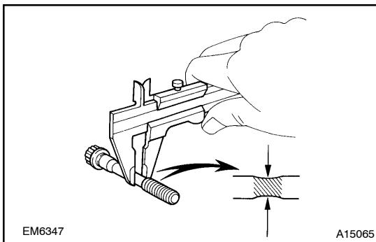
**24. INSPECT CRANKSHAFT BEARING CAP SET BOLT**
