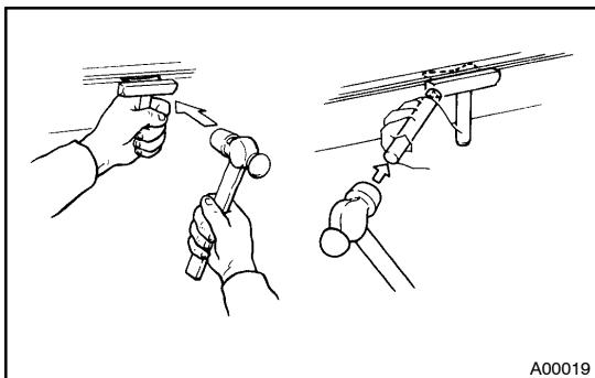
(b) Insert the blade of SST between the crank case and oil pan, cut off applied sealer and remove the oil pan.
