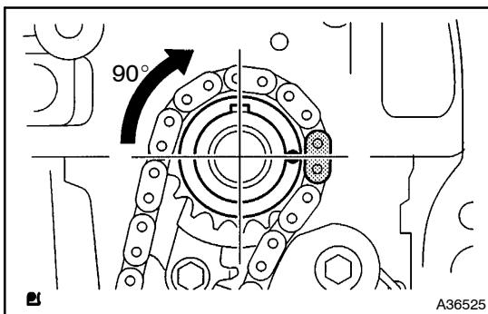
(i) Rotate the crankshaft counterclockwise 90°, and align the crankshaft key to the top.
