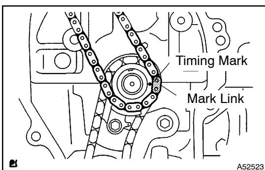
(b) Align the mark link (gold or orange colored link) with the timing mark of the crankshaft timing gear.
