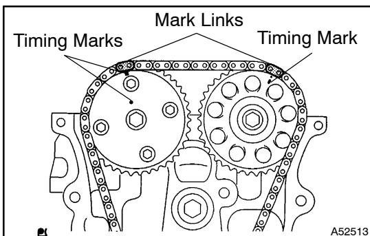
(d) Align the mark links (gold or yellow colored links) with the timing marks of the camshaft timing gear, and install the chain.
