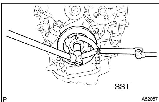
(b) Install the crankshaft pulley (TMMK made).
