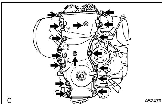
**29. REMOVE TIMING CHAIN OR BELT COVER SUB-ASSY**
