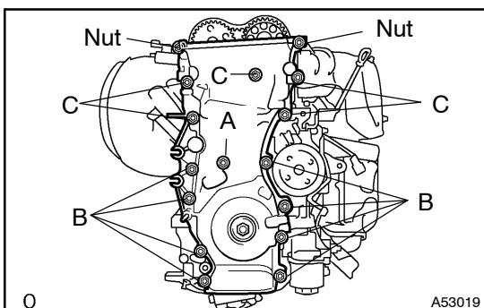
(d) Install the timing chain cover with the 14 bolts and 2 nuts.
