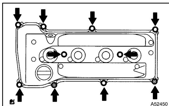
19. REMOVE CYLINDER HEAD COVER SUB-ASSY
