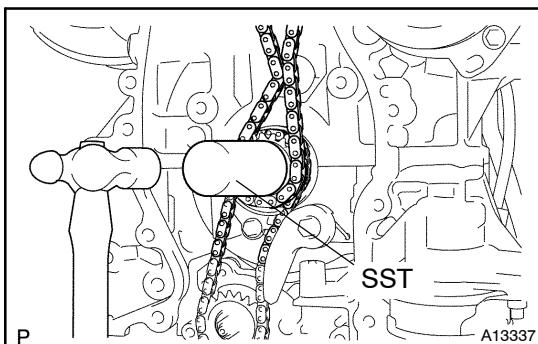
(c) Using a SST, install the sprocket.
