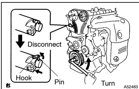
(c) Turn the crankshaft counterclockwise, and disconnect the plunger knock pin from the hook.
