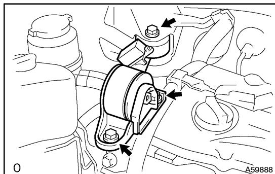
8. REMOVE ENGINE MOVING CONTROL ROD W/BRACKET
