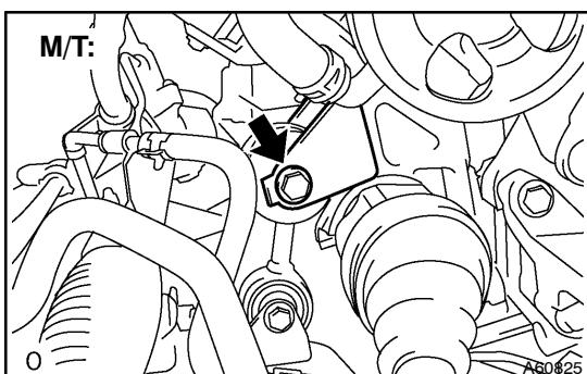
(e) Install the engine lateral control rod with the bolt (M/T).
