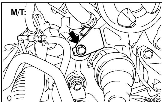
(c) Remove the bolt and disconnect the engine lateral control rod (M/T).
