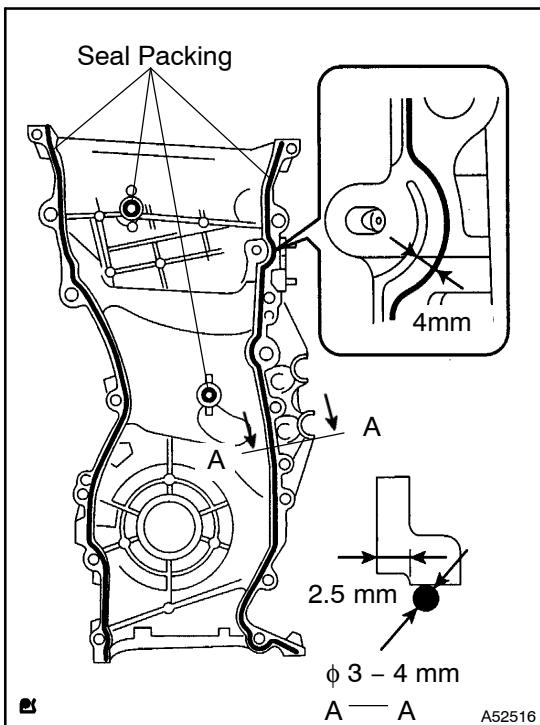
(c) Apply seal packing in the shape of bead (Diameter 3 – 4 mm (0.118–0.157 in.)) as shown in the illustration.
