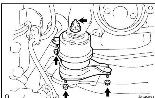
(e) Remove the 4 nuts from the engine mounting insulator RH.
