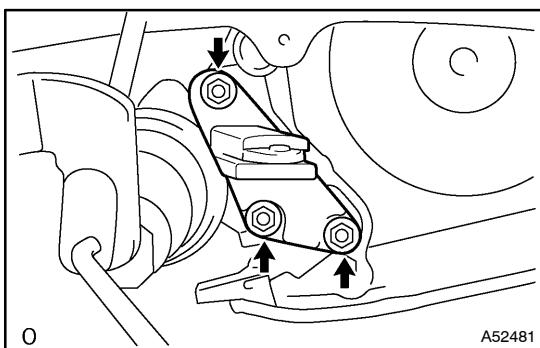
**43. INSTALL TRANSVERSE ENGINE ENGINE MOUNTING BRACKET**
