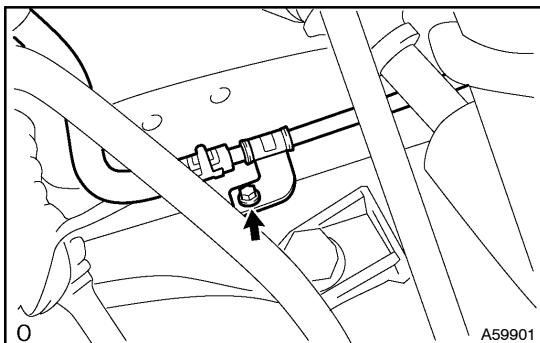
(c) Install the bolt and disconnect the steering gear return hose cramp from the frame.
