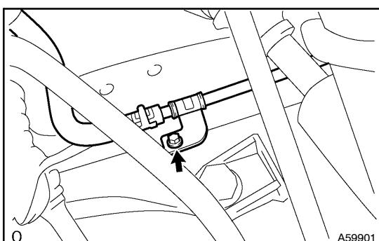
(d) Remove the bolt and disconnect the steering gear return hose clamp from the frame.
