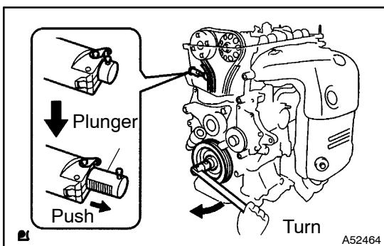
(d) Turn the crankshaft clockwise, and check that the slider is pushed by the plunger.
