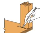
**4. Notch corners of plywood shelves.** Use a piece of 2x4 on each corner of the shelf, trace and cut to accommodate corner posts (only notch back corners of top shelf).
